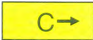
Runway Exit Sign
