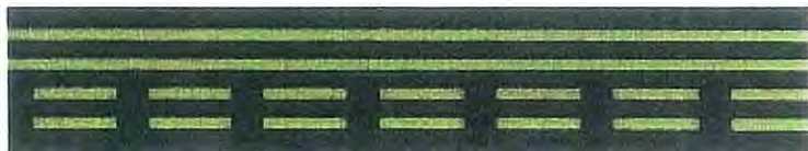
Runway Holding Position Marking
