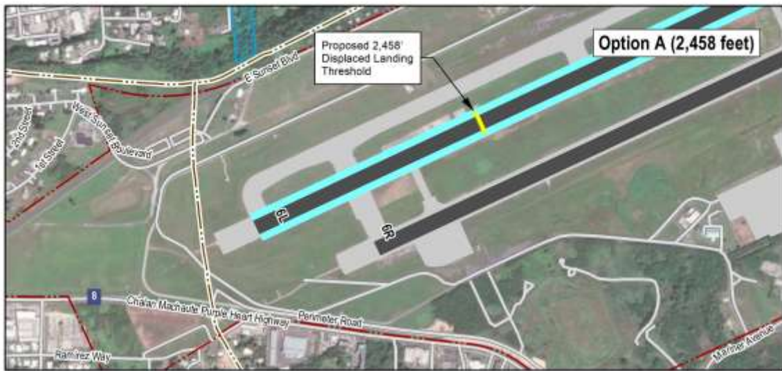
Figure 2-8. Landing Displaced Threshold Options for Runway 6L Source: GIAA 2024 Master Plan, 2025 Part 150 Noise Compatibility Study
