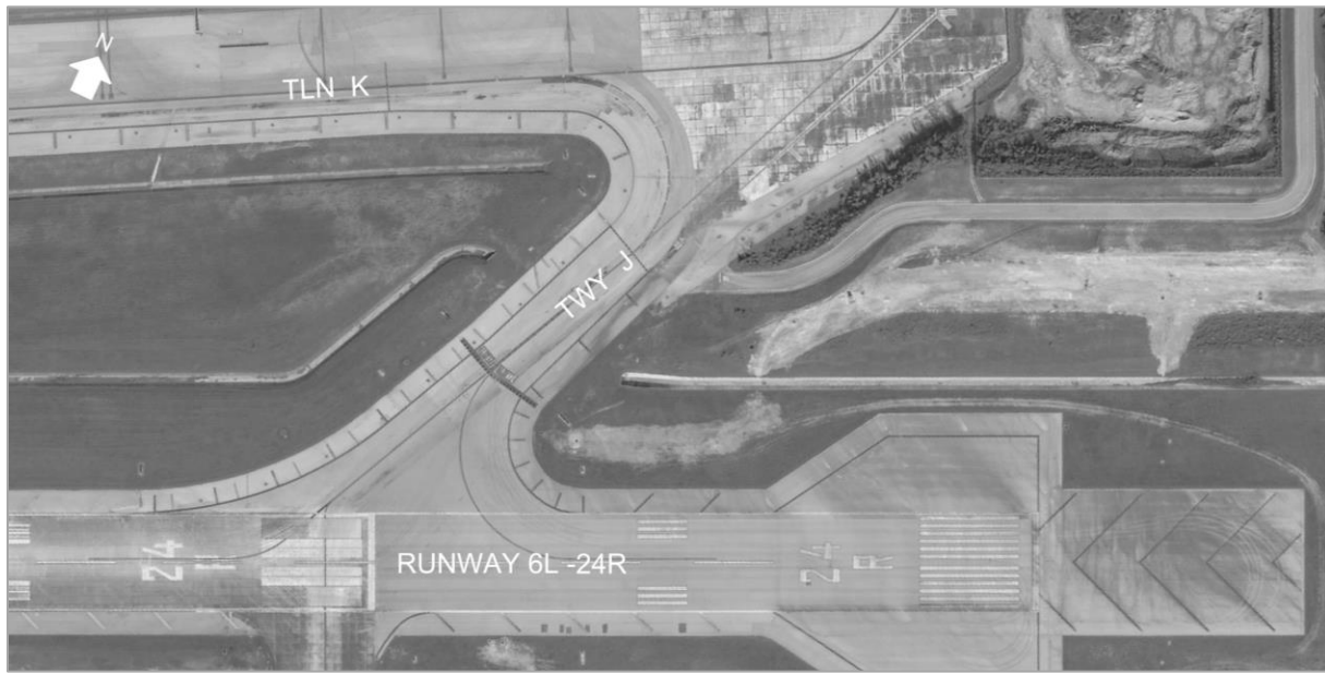
Figure 4-16. Problematic Taxiway Geometry – Taxiway Intersects at Other Than Right Angle, Direct Access to Runway, Short Taxi Distance, and Use of Runway as a Taxiway
